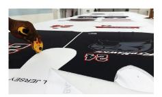
**03. FABRIC CUT AND SEW** Once the design has been "transfered" onto the substrate, the design is cut out.
