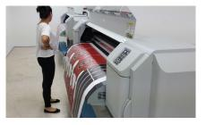
**O1. PRINTING** Unique sublimation dyes are transferred to sheets of "transfer" paper via liquid gel ink through a piezoelectric print head. The ink is deposited on these high-release inkjet papers.
